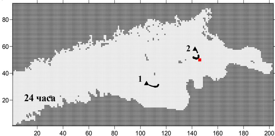
Figure 4.6 – Estimated grid area of the Gulf of Finland, the location of the points and the results of calculation of the oil pollution in 24 hours
