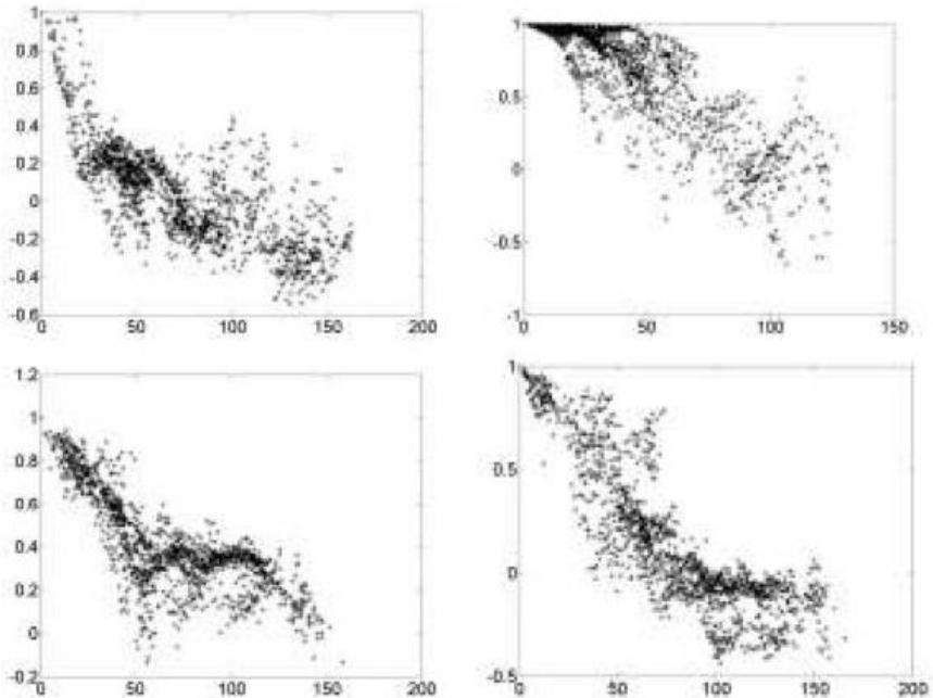
Figure 3.4 – Correlation coefficients between SST in the randomly chosen four points and the observational values in the other points. On the abscissa – distance in km, On the ordinate – correlation coefficient value
