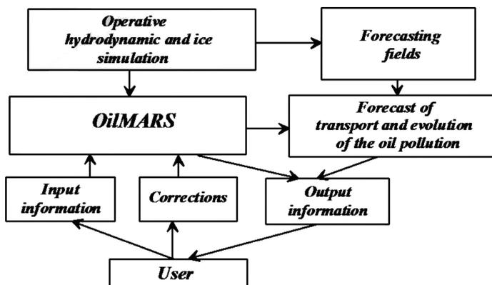
Figure 4.4 – Scheme of operational forecasting model of oil pollution
