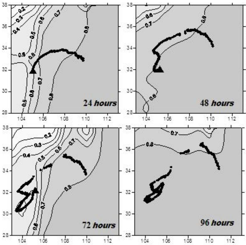
Figure 4.10 – Simulation example of oil pollution propagation in the winter at a point located in the central part of the Gulf of Finland. Isolines represent the concentration of ice (expressed in a decimal numbers)
