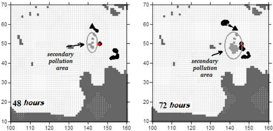
Figure 4.9 – Example of the oil pollution propagation simulation at. Contamination on the surface of the water is in black; secondary pollution is in grey
