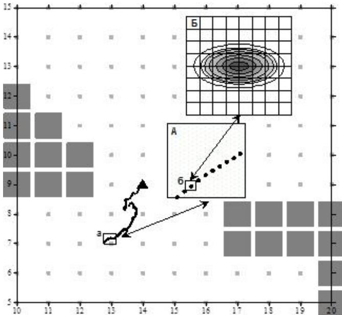
Figure 4.5 – Scheme of application of Lagrangian-Euler approach to the description of transfer and transformation of emergency oil spill. Areas marked with lower case letters correspond to the inserts marked with capital letters. On axes – grid coordinates
