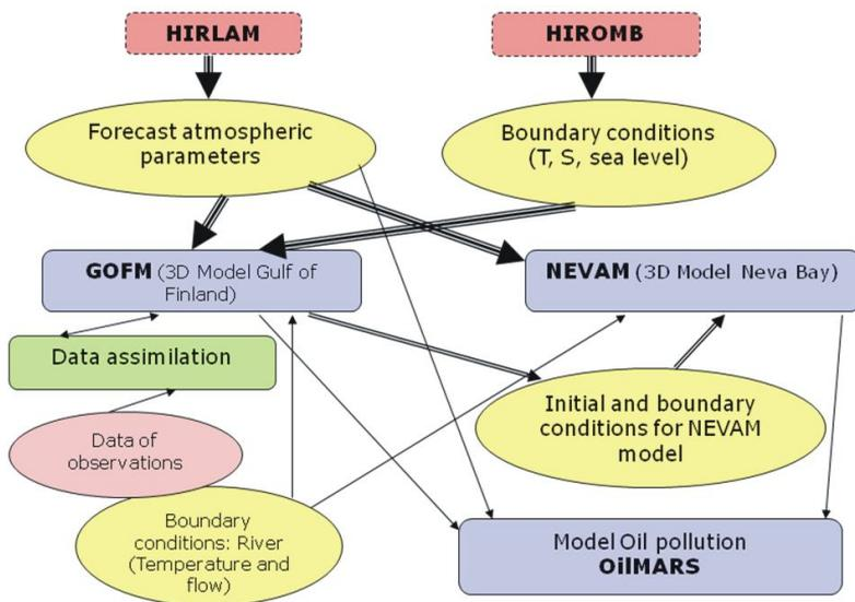
Figure 4.1 – Operational oceanographic forecasting system for the Gulf of Finland GULFOOS. The dotted line shows the planned, but still unrealized part of the system intended for SST assimilation
