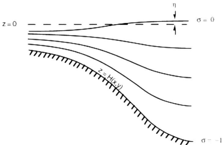
Figure 2.1 – Vertical structure of a model with  $\sigma$ -coordinate
