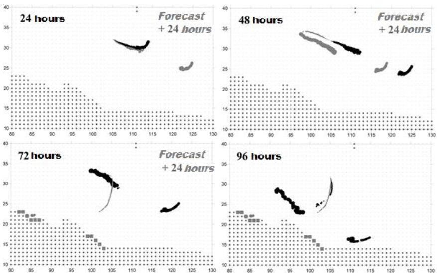
Figure 4.7 – Example of operational forecast calculating of the oil pollution propagation at the point 1. The “real” spill in shown in black and its forecast distribution for a day is shown in grey
